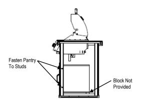
NOTE: Support the back end of your pantry insert with a 1 ¼" x 2 ½" x 30" block. Too much weight inside the pantry insert will cause it to bow and bend. Block NOT provided.
