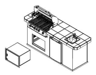
2. Fasten sides of assembled pantry insert to vertical studs inside island.
