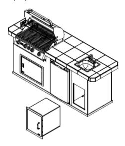
2. Fasten sides of assembled pantry insert to vertical studs inside island.
